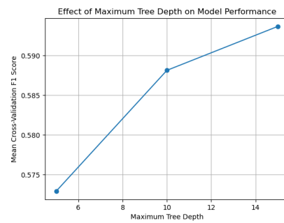
Fig. 19. Effect of maximum tree depth on cross-validation F1 score during Random Forest hyperparameter optimisation.
